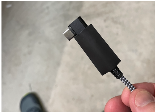
The 90° adapter with heat shrink tubing over the tape junction for extra security.
